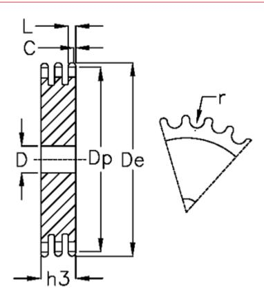
C = 2 D = 30 De = 700.6 Dp = 691.36 For chain size =  $3/4 \times 7/16$ For chain type = 12 B-3
